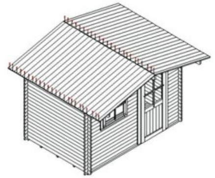
10. The roof assembling begins with the beams setting in the house triangle spots, the roof boards setting from front to back, bottom-up, windboard setting, lath under roofboards setting. Lath under roofboards will be sit under roof boarging panneling tying with these the cover edge board. The remaining space between the flatted annex-pair edge and the panneling profile can be closed using exterior silicone with adhesion to wood which will be applied before roof boarding panneling setting.
