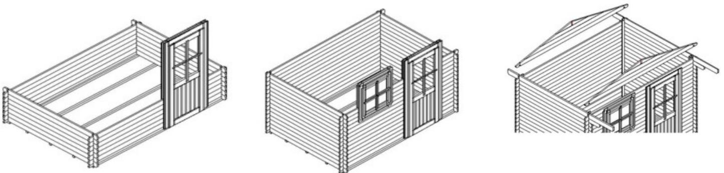
8. **The carpentry elements can be assembled in the same time with the walls assembling.** Their losing adjustment will be made after the roof assembling. Avoid using the doors and the windows before the final adjustment.
